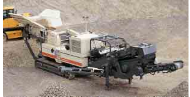
Lokotrack LT96S jaw plant with a detachable screen.
