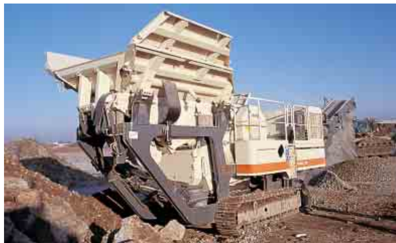
Another unique Lokotrack LT96 feature is the automatic locking mechanism for the feeder, cutting the time needed to prepare for transportation.
