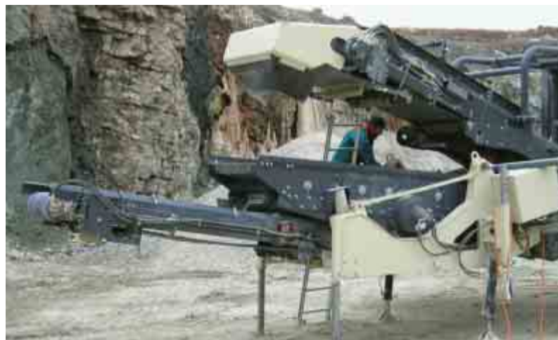
The screen of Lokotrack LT1213S can be opened easily for servicing and screen mesh change using the hydraulic system.
