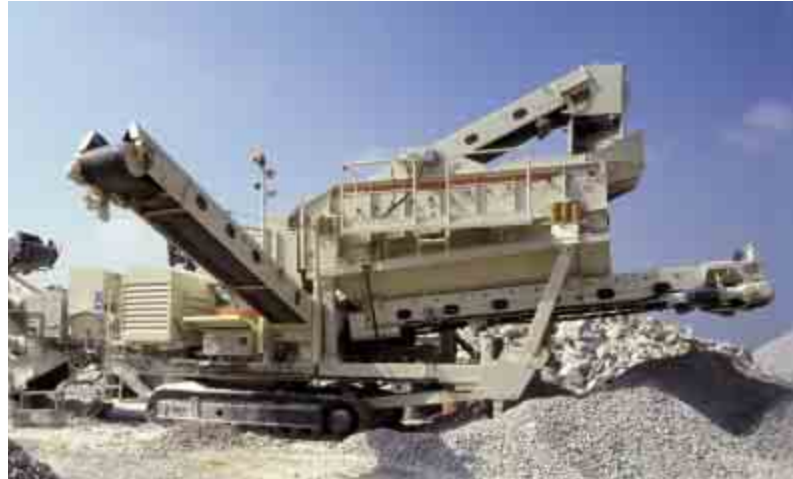
LT1100 can be transported easily between sites as a single unit on trailer.
