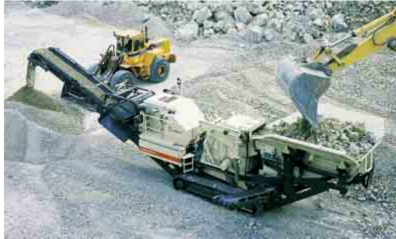
According to the application, Lokotrack LT1110 can be equipped with 5m 3 or 8m 3 sized feed hopper.
