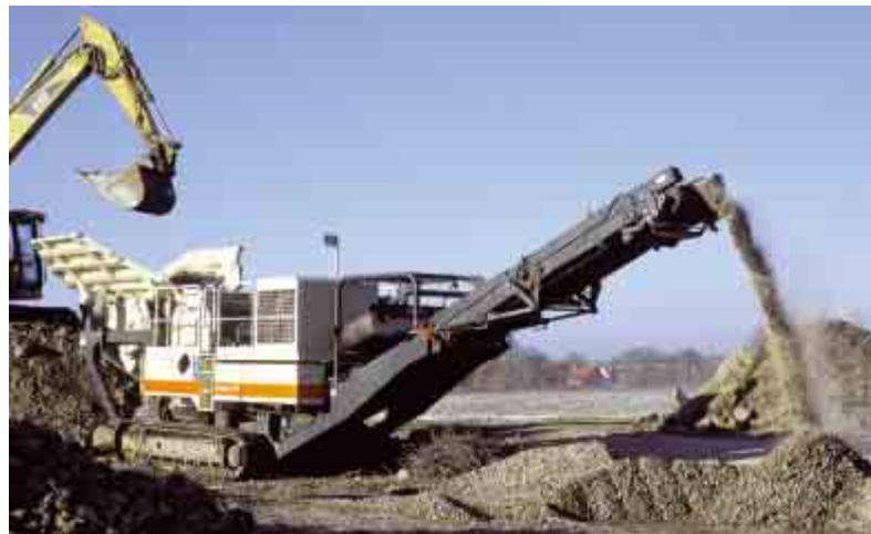
The sturdy and long main conveyor can be equipped with an optional magnetic separator for recycle applications.
