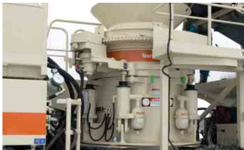
LT200HP is built around the proven and popular HP200 cone crusher.
