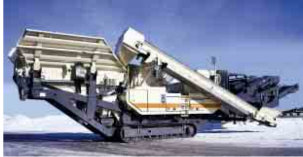
Lokotrack LT1110S impactor plant with a detachable screen.
