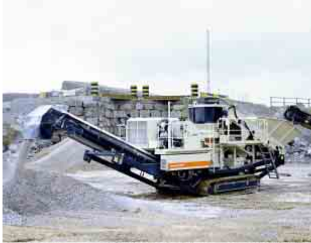
Lokotrack LT200HP cone plant.
