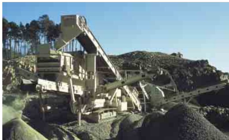
The three-deck horizontal screen has a screening area of 8 m 2 per deck.
