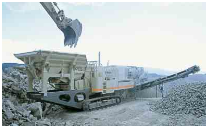
The Lokotrack LT105S side conveyor is easily tilted for transport.
