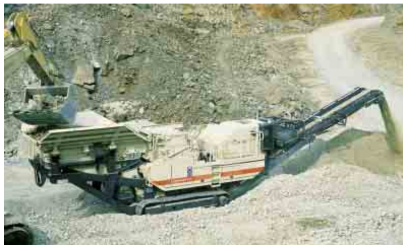
New design using separate elements result in lower operating noise levels.
