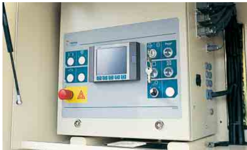
The revolutionary IC500 intelligent controller controls the whole crushing operation and gives real time crushing information about all the main functions.
