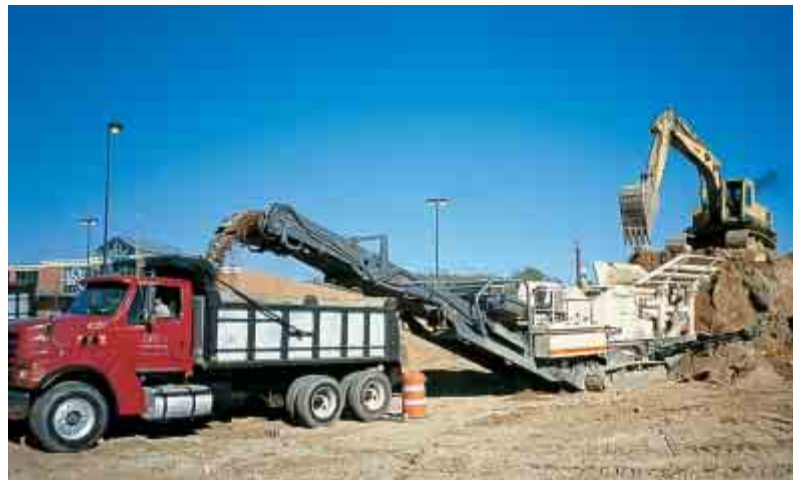
Lokotrack LT105 equipped with an extra long 12 metre conveyor crushing in the USA.
