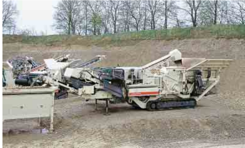
When used at closed circuit, the Lokotrack LT1213S produces one, exactly calibrated end product.
