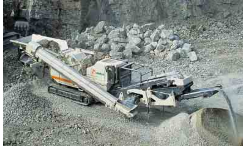
Thanks to the IC500 intelligent controller, unmanned operation of Lokotrack LT1110S is well possible.
