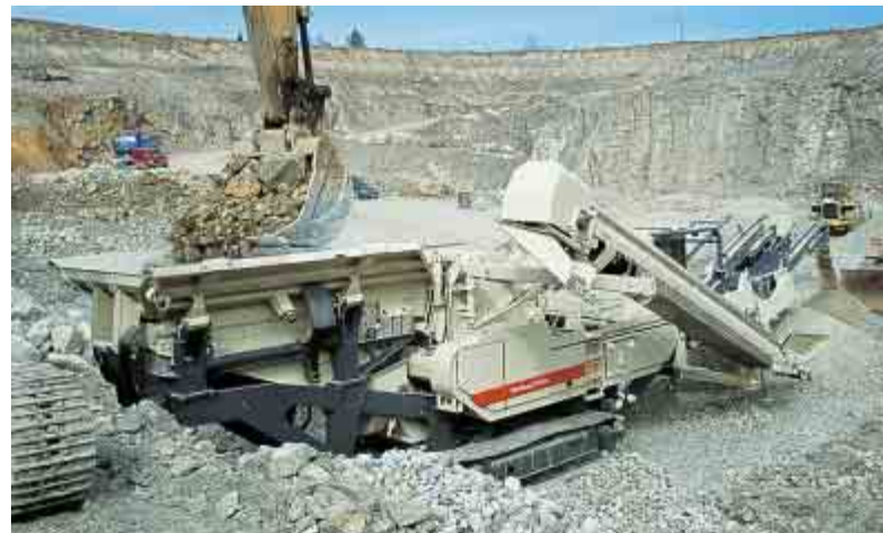
Lokotrack LT1110S crushes and screens all medium hard stone types and mineral based demolition materials.
