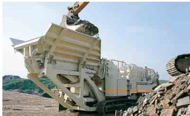
The sturdy feed hoppers in all Lokotrack LT Series mobile crushing plants are manufactured from high-quality wear resistant steel.
