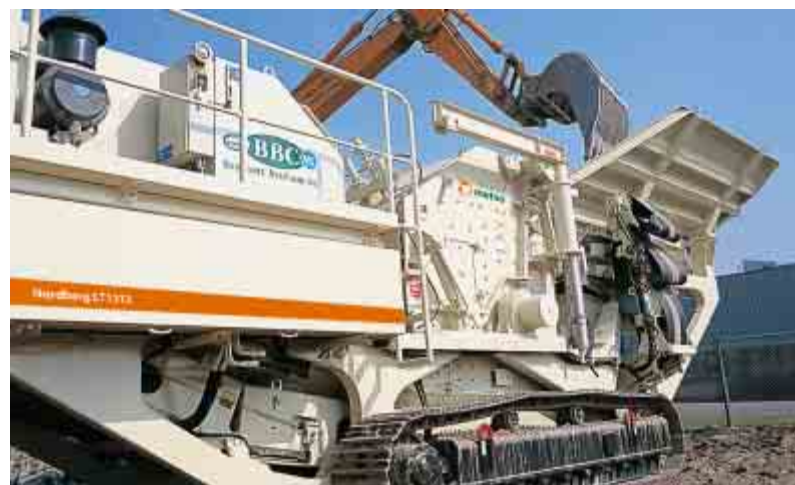
The new, Nordberg NP1213M impact crusher has been developed for the Lokotrack LT1213 mobile crushing plant.
