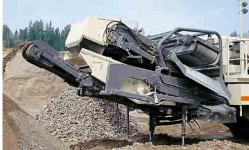
The screening unit can be disconnected in minutes allowing the Lokotrack LT105S to be used as a normal primary crushing unit.
